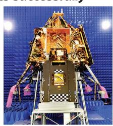
test, launcher compatibility, antenna polarisation of all RF systems, standalone auto compatibility tests for orbital and powered descent mission phases, and Lander and Rover compatibility tests for post landing mission phase were ensured.
